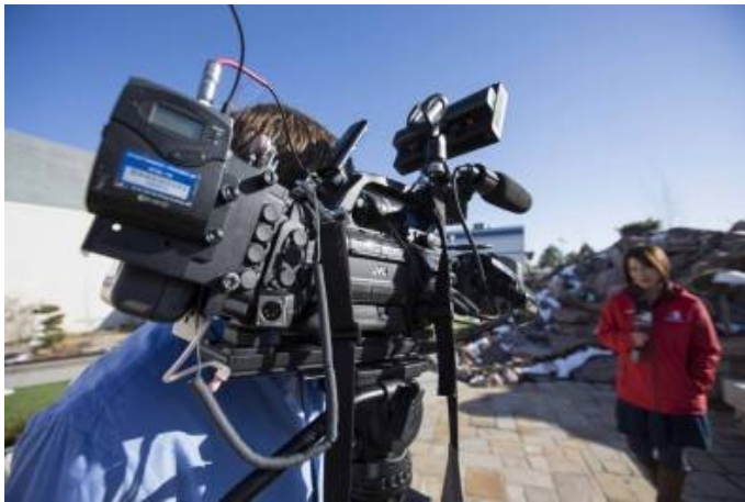
Salt Lake City station KTVX, is using six JVC GY-HM890 ProHD shoulder-mount camcorders in conjunction with the JVC BR-800 ProHD Broadcaster server (powered by Zixi technology) to produce live ENG reports from the field.
